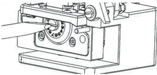
1. Unscrew the fastening screw of the blade, turning in a counter-clockwise direction with a screwdriver. Rotate blade by one position to the next number (original number on blade plus one), then tighten screw.
