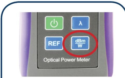
3. On the OPM, press the “dBm/W” button until dBm is the unit listed to the right of the main screen read-out (see step 1B image).
