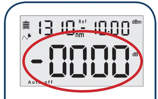
Once cable(s) are connected between OLS and OPM units, press and hold “REF” button for two seconds. OPM should now read 0dB.
