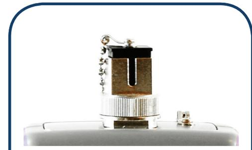
4. Plug REFERENCE cable into OLS. **Note: Do not look into laser while unit is on.**
