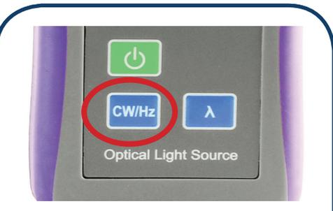
2. On the OLS press CW button until dashes display in lower right of the screen (see step 1A image).
