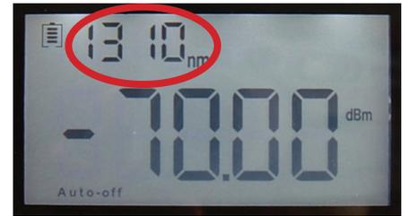
B. The OPM should be set to same wavelength as the OLS unit. Press the wavelength button until desired value appears.
