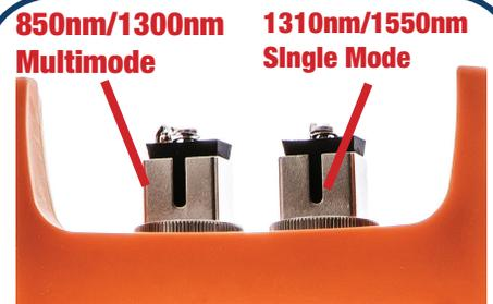
4. Plug REFERENCE cable into the appropriately labeled port on the OLS. SC testing: single-ended testing/ 1 cable. LC testing: double-ended testing/ 2 cables.
