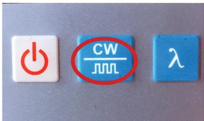
2. On the OLS press CW button until 0Hz displays in upper right of the screen (see step 1A image).
