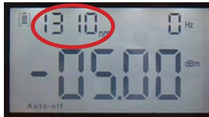
A. Wavelength on the OLS is displayed in the upper left corner of the screen. Set to desired value (press wavelength key.) Hz (upper right) will have a numeric reading when the laser is on. \*Dashed lines (----) indicate laser is off.
