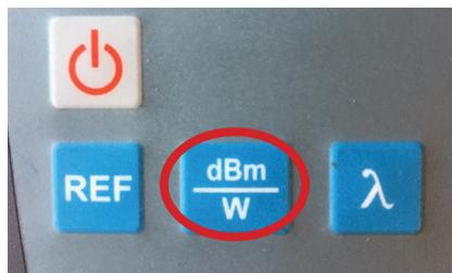
3. On the OPM, press the “dBm/W” button until upper right portion of screen is blank and dBm is listed to the right of the main screen read-out (see step 1B image).
